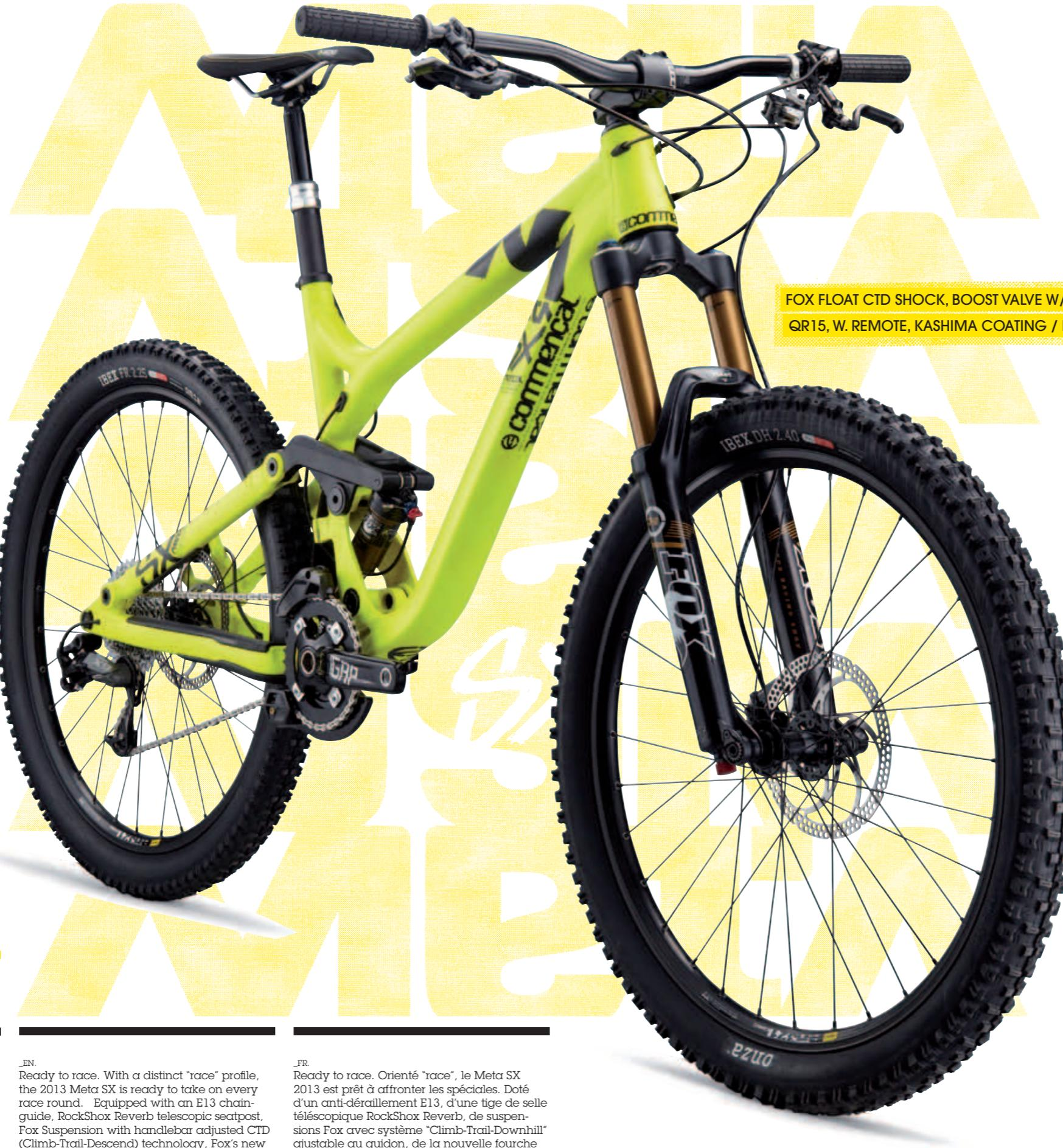
FOX FLOAT CTD SHOCK, BOOST VALVE W/REMOTE, KASHIMA COATING / FOX 34 CTD FIT FORK, TAPERED, QR15, W. REMOTE, KASHIMA COATING / FORMULA RX 12 DISC BRAKES / ROCKSHOX REVERB SEATPOST
