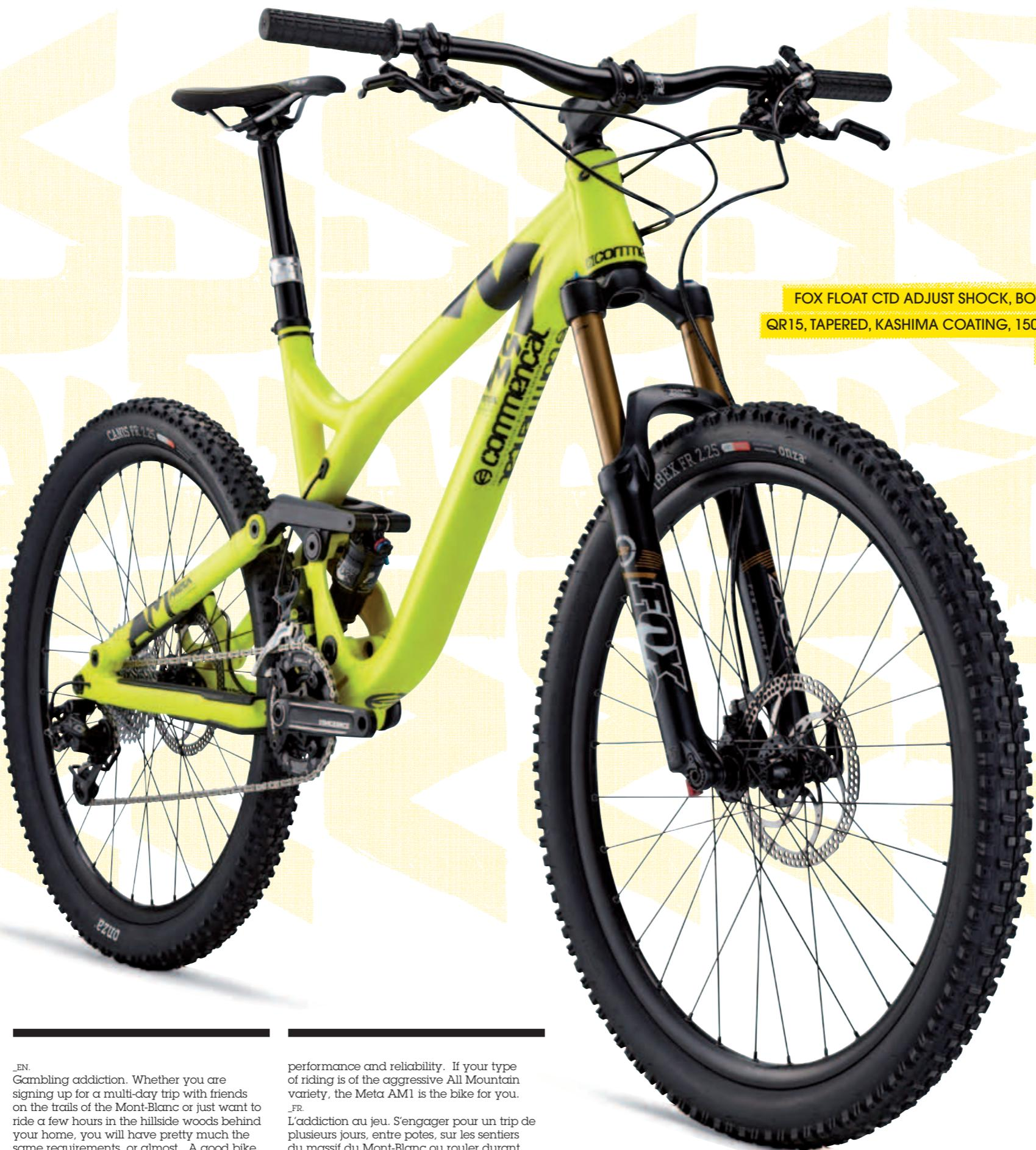
FOX FLOAT CTD ADJUST SHOCK, BOOST VALVE, KASHIMA COATING / FOX 32 FLOAT CTD ADJUST FORK, QR15, TAPERED, KASHIMA COATING, 150MM / SRAM X0 2X10 SPEEDS TRANSMISSION, TYPE 2 REAR MECH / FORMULA RX 12 DISC BRAKES / ROCKSHOX REVERB SEATPOST
