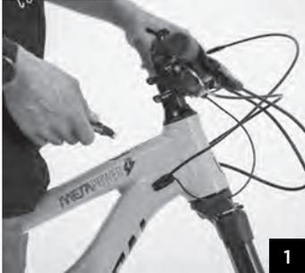
If preferred, you can adjust your handlebar height by modifying the spacer stack. To do so, unscrew and remove the topcap. Then, untighten the stem bolts. Remove the stem and adjust the spacer stack to change height.
