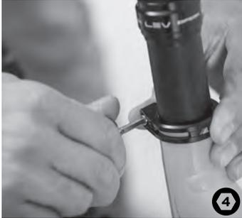
To adjust your saddle height, untighten the seat clamp (by hand or with an allen key), adjust the height and tighten the seat clamp.
