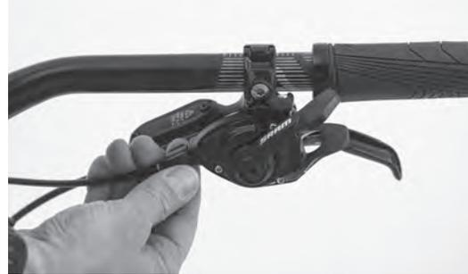
Once your limit screws are set, you have to adjust the cable tensioner. Try shifting through the gears:
