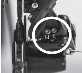
The limit screws prevent your chain from exceeding the limits of the cassette. You have one screw controlling the higher limit (H) and one screw for the lower limit (L). The higher limit corresponds to the smallest cassette ring while the lower limit corresponds to the biggest cassette ring. Adjust so that you achieve the correct limitation without compromising gear range.
