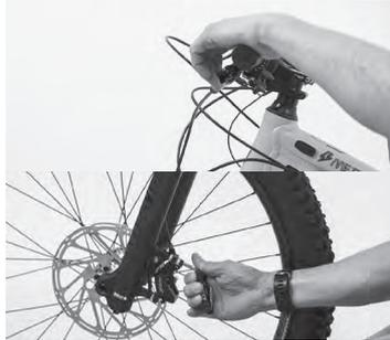
Whilst holding the brake lever, tighten the caliper bolts.
