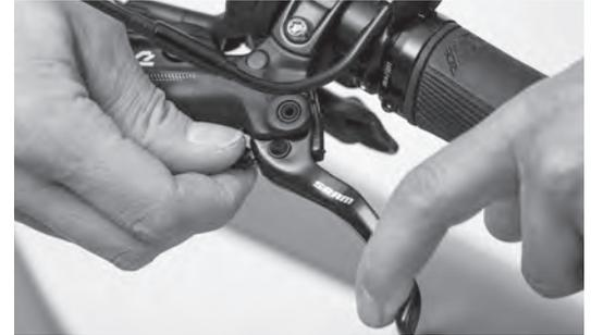
You can adjust the reach of the brake lever. Simply turn the fine adjuster found on the brake lever. This can also be in the form of an allen key bolt.
