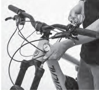
It is very important to set up your suspension corresponding to your weight. Regulate the pressure of the suspension with the high pressure pump.
